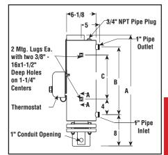
**Vessel** — Pipe body and nozzles are ASTM A53B carbon steel pipe. The end disk is ASTM A516 Grade 70 carbon steel plate. Provided with thermal insulation and painted sheet metal jacket.
