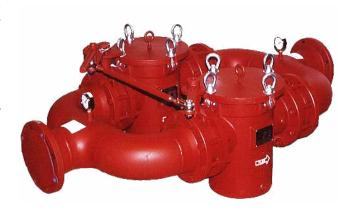
The Series 530/531 is a compact unit, in-line inlet/outlet connections, which enables easy piping and variable strainer placement. Chamber change over is accomplished quickly and easily. A single lever controls the positive sealing butterfly valves, changing the fluid flow.
